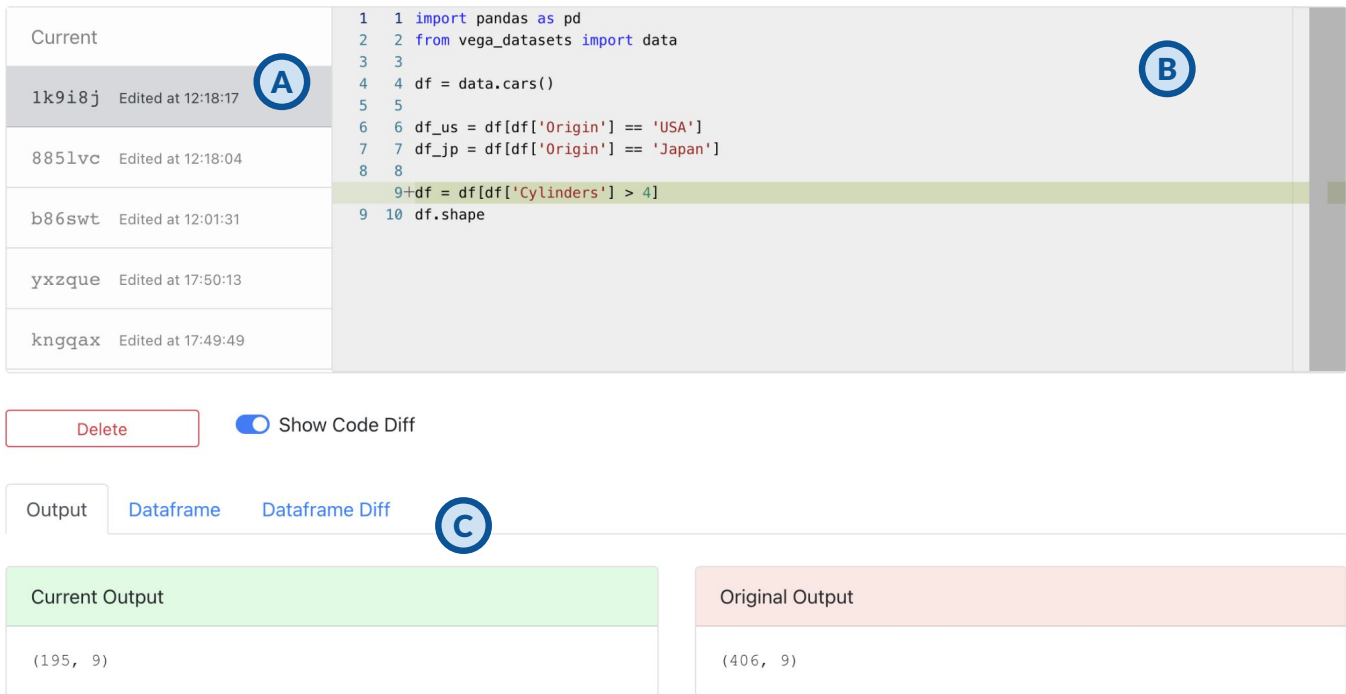
Figure 2: We integrate DITL into a simplified data science programming environment that allows data scientists to edit code, inspect data tables, and compare different data tables. This interface shows that the user is browsing a snapshot tagged 1k9i8j where the edit took place at 12:18:17. (A) Users are able to navigate among saved snapshots, compare code differences and output differences, or switch to the current code editor; (B) Users can edit code in the current code editor which automatically saves a new snapshot upon successful execution, or view code changes in a snapshot; (C) Users can switch between the output panel, the data panel panel, and DITL.
